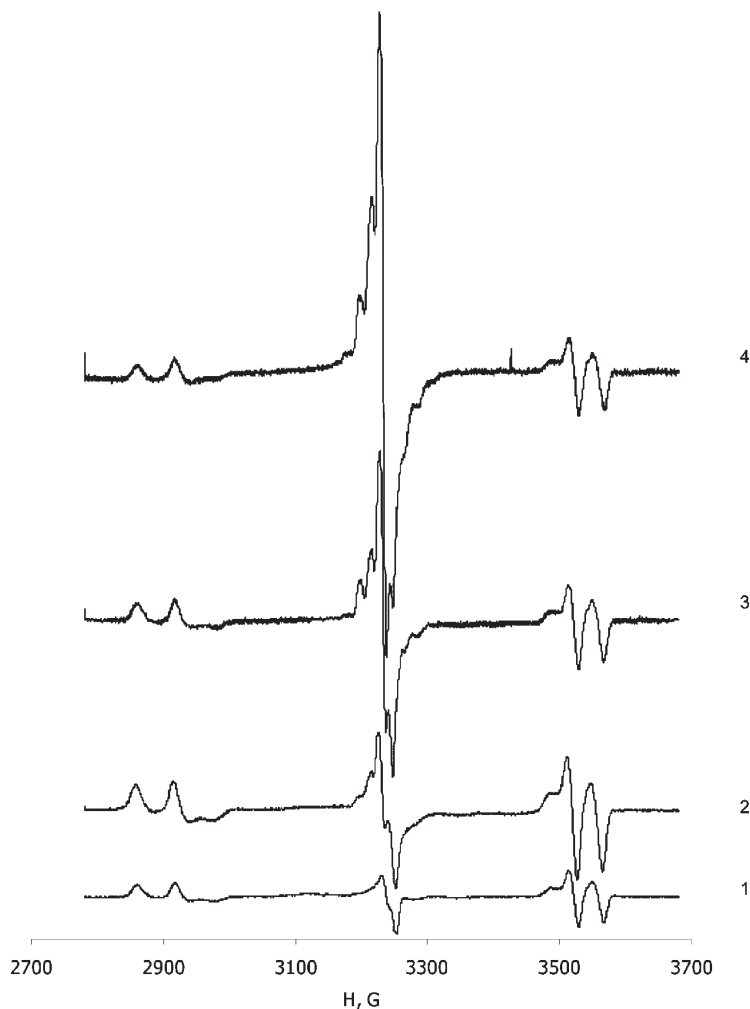
FIGURE 1 The ESR spectra of the samples of triple system Ag-CCl 4 – 4-n-pentyl-4'-cyanobiphenyl obtained during low temperature vacuum cocondensation, containing different proportion of the components: 1-1:0:100, 2-1:1:100, 3-1:3:100, 4-1:10:100.
